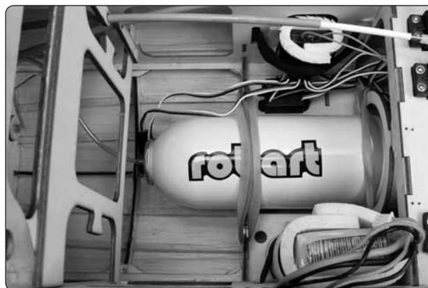
❑ 1. If installing the pneumatic retracts attach a 12" (305 mm) piece of airline tubing to the pressure tank. Insert the pressure tank into the fuselage. A couple of dabs of silicone sealant such as Shoe Goo® can be applied to the pressure tank supports to hold the tank in position but still allow it to be removed if necessary. Secure the pressure tank to the supports with four #64 rubberbands.
