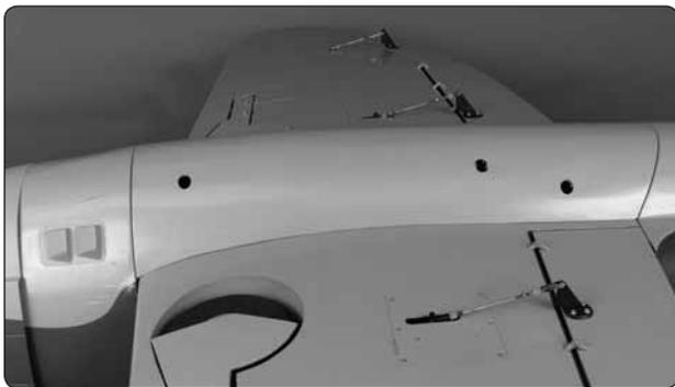
❑ 9. Test fit the wing on the fuselage and make any adjustments required to get a good fit between the wing and fuselage. This may require some sanding of the wing dowel holes in the front of the fuselage.
