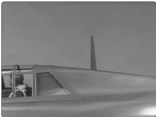
❑ 9. Insert the antenna mast in the top of the fuselage. The mast is held in place with magnets.
