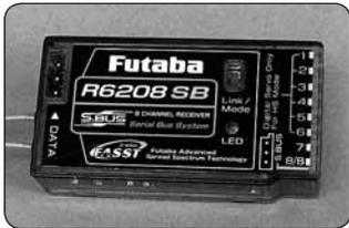
There are many choices for the S. Bus receivers; some are tiny 3 port receivers with others being up to 8 channels. The 8 channel inputs can be used as you would
