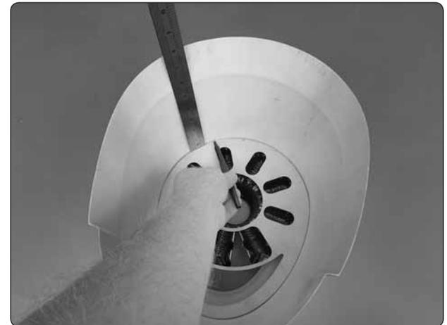
❑ 13. Test fit the radial engine assembly in the cowl. Position it so it is centered and equal distance from the edge of the cowl. Mark the location on the inside of the cowl. This will help you reposition the engine once you have applied epoxy to the engine assembly. Use masking tape to hold the dummy engine in position and test fit the cowl on the fuselage.
