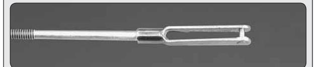
This is what a properly soldered clevis looks like – shiny solder with good flow, no blobs and flux removed.
