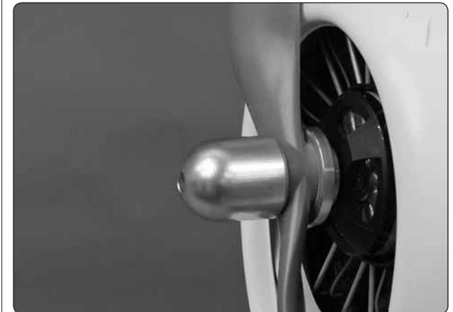
❑ 5. Secure the spinner cone to the spinner adapter with a 10-32 x 1" socket head cap screw (not included).
