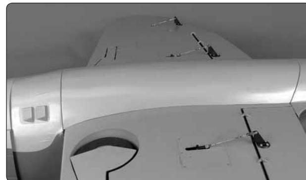
❑ 5. Glue the belly pan to the wing using 30-minute epoxy. Make sure that the belly pan is tight against the bottom of the wing and centered between the fuselage. Wipe off any excess epoxy before it cures.
