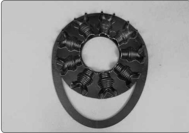
❑ 6. The plywood engine frame can be painted black. Use 6-minute epoxy to glue the plastic radial engine to the plywood engine frame. Align the radial engine with the embossed circle on the plywood frame.
