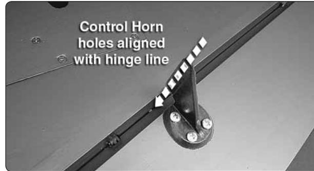
2. Position the control horn so that it is inline with the pushrod and over the plywood mounting plate. The pushrod holes in the control horn should be aligned with the hinge line of the aileron. On the aileron, mark the four mounting holes. Remove the control horn and drill a 5/64" [2mm] pilot hole at each mark. Do not drill completely through the aileron. Attach the control horn using four #4 x 1/2" [12.7mm] sheet metal screws. Use thin CA to harden the holes.
