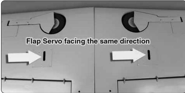
1. Install the flap servos following the same procedure used to install the aileron servos. Note that the flap servos face the same direction.
