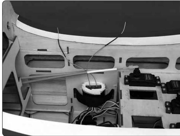
□ 13. Glue the plywood pushrod support so that the pushrod is inline with the servo arm and on the outside of the aft fuel tank support.
