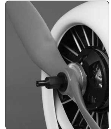
❑ 4. **APC Electric Propeller:** Enlarge the propeller shaft hole to 10mm using a metric prop reamer or a size 'X' drill bit. Trim 1/4" [5 mm] from the end of the spinner adapter (GPMQ4590 not included) so that the adapter is 1-1/4" [32 mm] long. Install the propeller on the motor shaft and secure it with the spinner adapter and washer.
