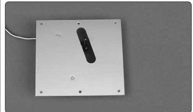
5. Drill 1/16" [1.6mm] holes through the blocks at the two hole locations on the top of the aileron servo hatch. Install two #2 x 3/8" [9.5mm] flat head sheet
