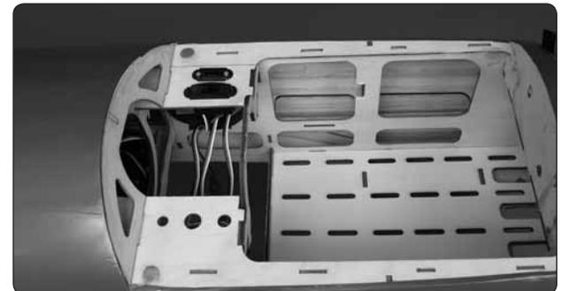
❑ 4. Mount the receiver on/off switch and the charge receptacle in the tray under the battery hatch.
