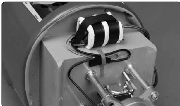
❑ 19. Place the ignition module on a piece of R/C foam rubber (not included) and secure it to the top of the firewall box with hook and loop material. The
