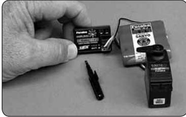
Once programmed the servo will operate as required regardless of which lead it is plugged into. Do this for all of the servos that you want to operate on
