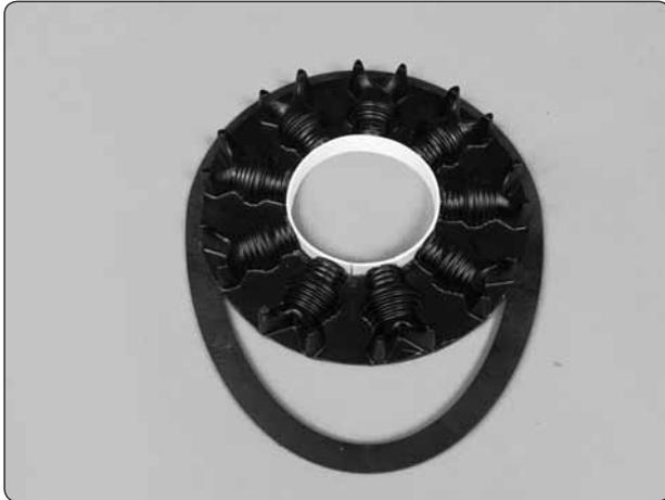
❑ 8. Place the assembly on a flat surface. Position one of the 7/8" x 12" (22 x 300 mm) plastic strips inside the hole and cut it to length. With the plastic strip against the flat surface, glue it to the plywood frame and the radial engine.
