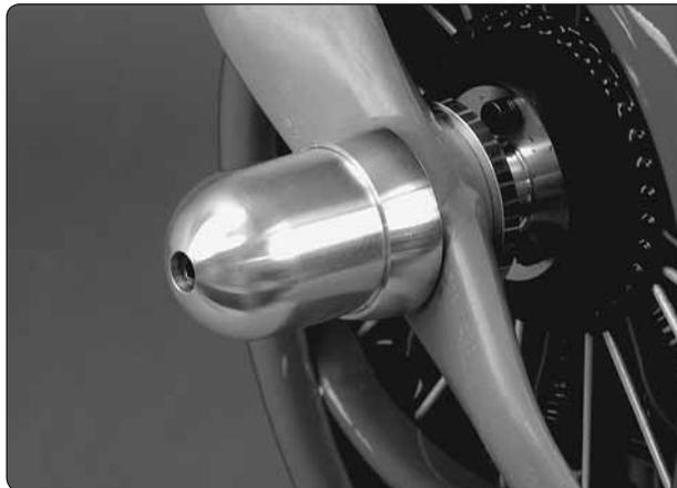
❑ 3. Install the prop hub cone on the engine using a M5 x 50mm socket head cap screw. Use a drop of threadlocker on the threads.
